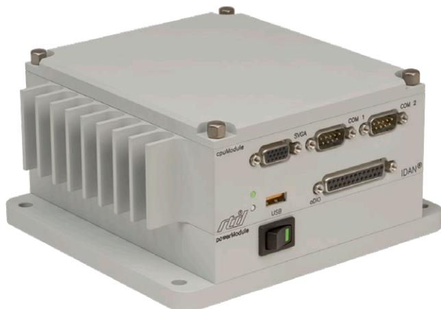
RTD's off-the-shelf IDAN® eBuild™ systems offer rapid up-time for system development and deployment. These pre-configured starter systems include a CPU and power supply, and can be expanded to include additional peripheral modules based on application needs.
