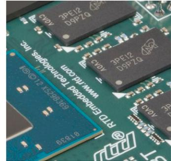
*RTD's rugged, single board computers feature surface-mounted RAM soldered directly onto the board to maximize reliability in extreme temperatures, and in high shock and vibration environments.*
