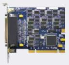
**BlueStorm/SP** is a high-speed multi-port adapter which offers 8 ports of RS-232/422/485 connectivity.
