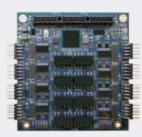
**Xtreme/104-Express Opto** is a PCle/104 serial card with 3 kV optical isolation for rapid data transfer and high reliability.
