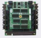
**FreeForm/104 Daughter Board** is a FreeForm/104 adapter board that enables users to capture and process synchronous and asynchronous RS-232 or RS-422/485 serial data with customizable FPGA implementations.
