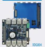
Xtreme/GbE Managed Carrier **Ethernet Switch** provides Carrier Grade Ethernet switching capabilities in an extremely small embedded form factor
