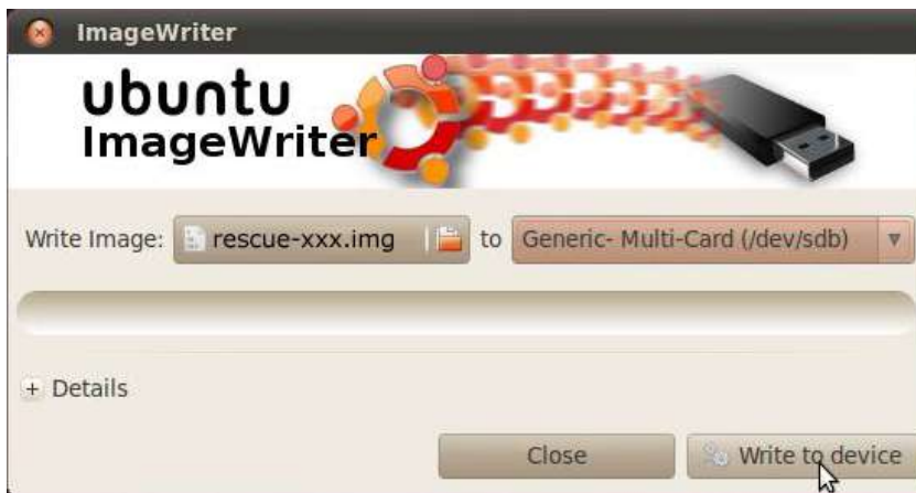
Figure 29: Select the downloaded image and destination (SD-card in your computer), click write to device
