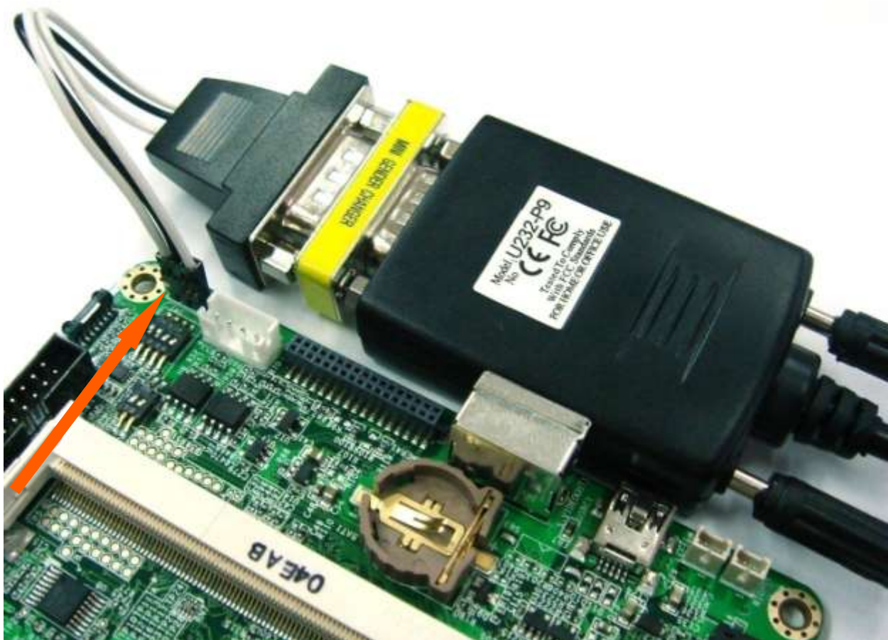
Figure 36: The cable (RS-232 to USB) with yellow mini-gender-changer-block connected to the UART1 (5) connector (see orange arrow for position of the white dot)
