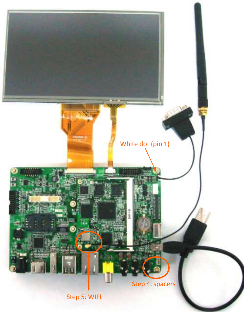
Figure 4: Step 3a - Connect the RS-232 serial console cable as on the picture above. (Note: RS-232 serial console cable might need a gender changer when connected to, for example, a null-modem. One can also reverse the connected cable)
