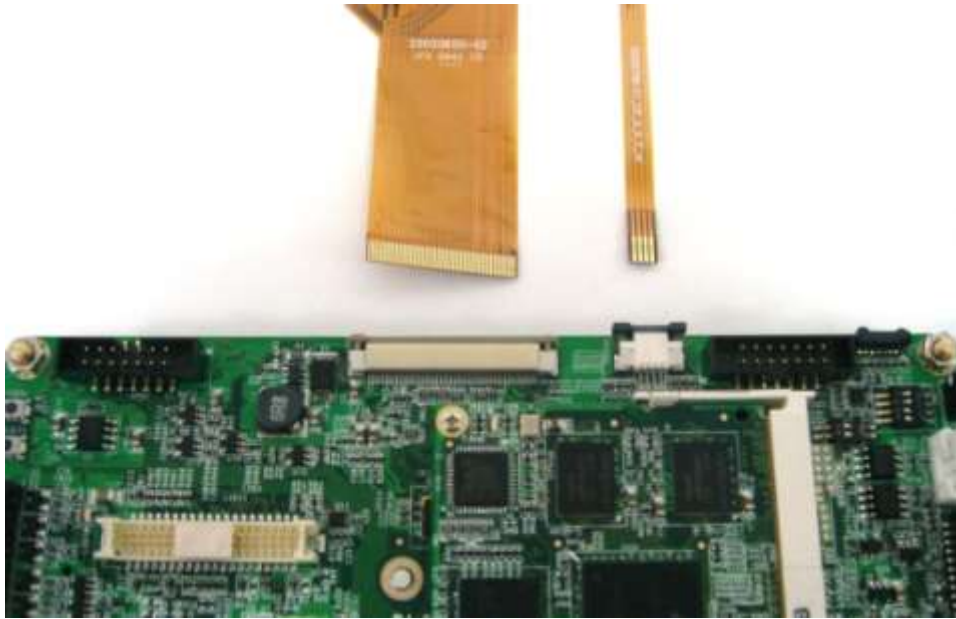
Figure 2: Step 2a - Pull the connector, on the topside of the PCB, sideward open with your nail.
