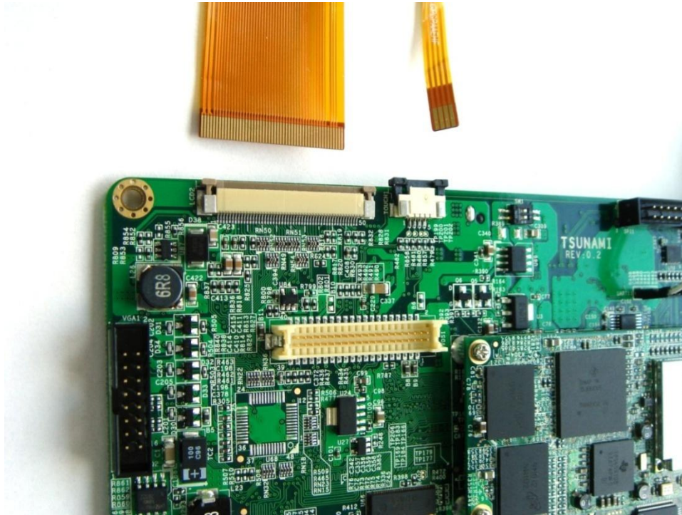
Figure 2: Step 2a - Pull the connector, on the topside of the PCB, sideward open with your nail.
