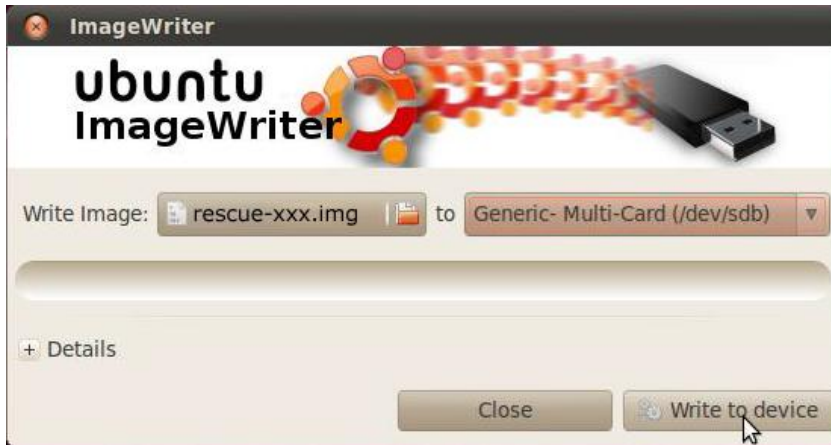
Figure 28: Select the downloaded image and destination (SD-card in your computer), click write to device
