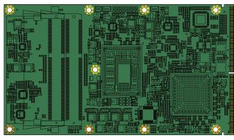
Intel QM77 with 3rd generation i3/i7 Core BGA mounted ultra low voltage processor
