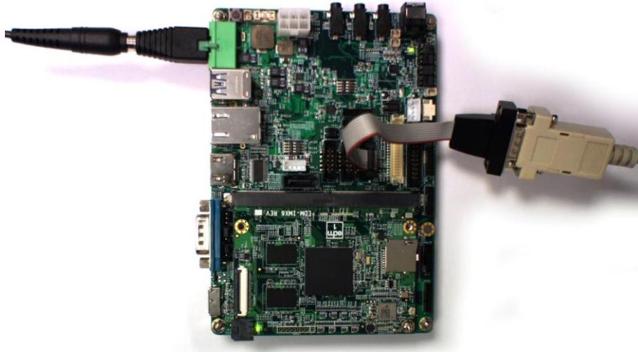
Figure 12: The terminal cable connected with the DE9 cable to the COM1 (UART1) connector.
