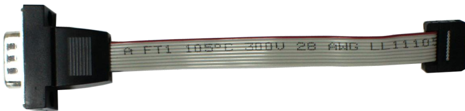
Figure 31: DE9 cable for the CAN BUS1 connector
