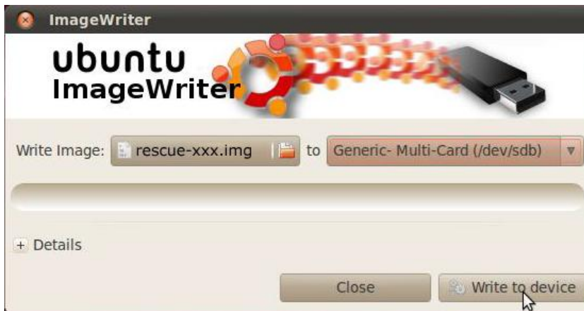
Figure 32: Select the downloaded image and destination (SD-card in your computer), click write to device
