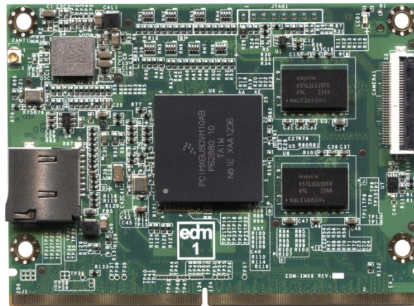
Figure 1 - EDM Module Marking Example
