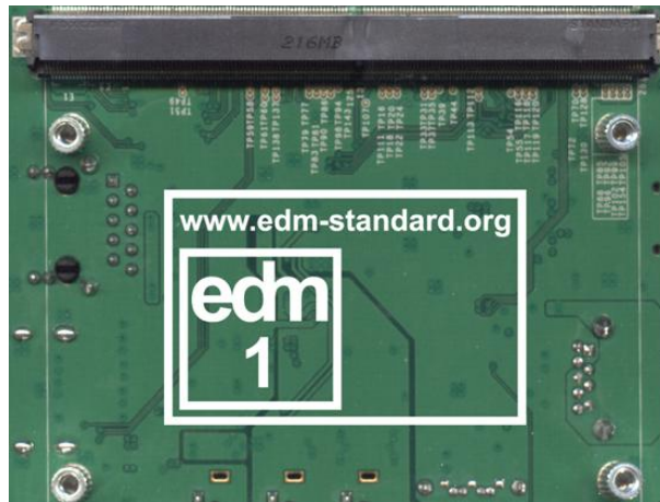
Figure 3 - EDM Carrier Board Marking Example
