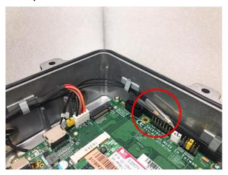
Step 7 Connect the SMA cables to I-PEX connector of LTE Module and install LTE Antennas. And please do not place antenna cables on the top of PCI Express mini card, in case the SMA cables would loose.
