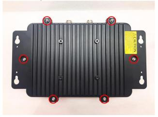
Step 3 Remove the bottom cover, and locate the PCI Express mini card slot on the board.
