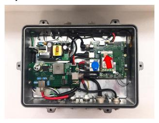
Step 5 Press it down gently, but firmly, and then secure the PCI Express mini card to the carrier by tightening up the one M2\*5L screw to the marked position.
