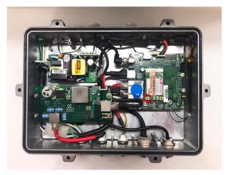
Step 6 Find the SMA cables from the adhesive backed cord clip attached at the chassis as picture below.
