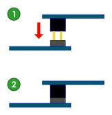
**Step 4**Secure the EPIA-P720-A I/O module with two screws.
