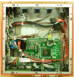
Step 2: Fasten the four HDD screws and black damper, and then you can put the HDD on the opposite side for screwing it up.
