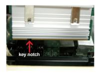
11. Attach another thermal pad onto the top of the heat spreaders.
