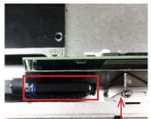
Adjust this iron to make space for the USB drive installed
