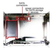
8. Connect the SATA signal cable(s) and power cable(s).
