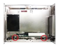
3. Install an USB drive to one of the internal USB ports.
