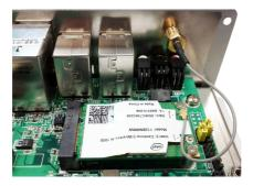
7. Pull the other end of the RF cable, a SMA connector jack, through the antenna hole. Be sure to meet the flat side of the antenna hole so the connector jack won't get stuck.
