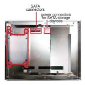
6. For the 2nd storage bracket: Assemble another HDD/SSD storage device to the storage bracket.
