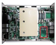
The MiniCard socket's connector has a break.
