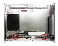
Install an USB drive to one of the internal USB ports.
