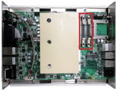
The SO-DIMM sockets are vertical type, and each socket has two latches for fixing the memory modules. The memory module can only be installed by one direction due to the key notch.
