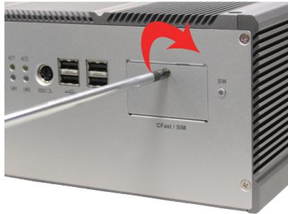
6. To remove the CFast card or SIM card, follow step 1, 2 and 3 above. And then push-release it from the slot.
