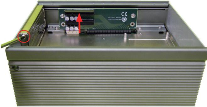
2. And penetrate through the hole on case side with screwdriver to remove lower bracket and install PCIe card.
