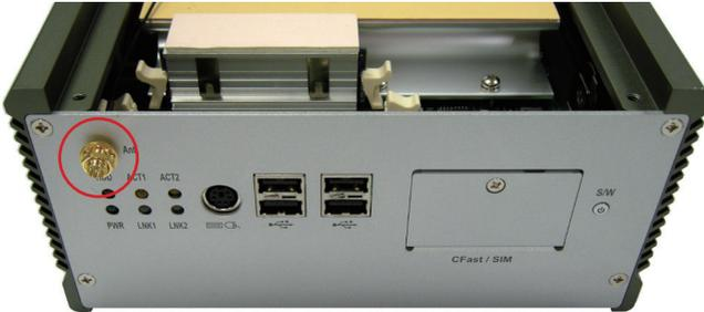
7. At the end, screw antenna into the SMA connector jack and adjust antenna angle for better signal.
