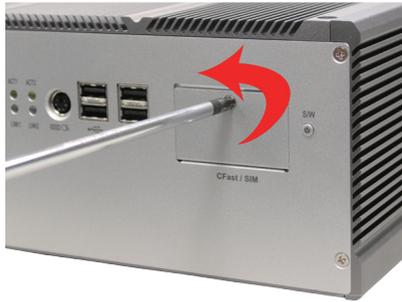
4. Insert your CFast/SIM card into the slot according to the illustration that you find close to the card door.
