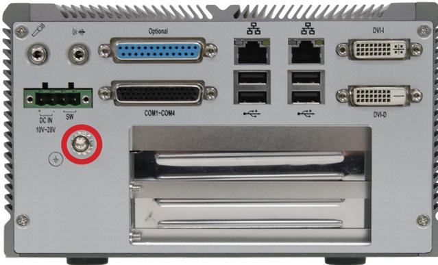
1. See the figure above. Remove the ground screw located on the rear panel.
