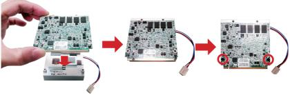
Confront the CPU board's edge connector with the carrier board's MXM connector. Align the CPU board edge connector notch with the MXM connector break.
