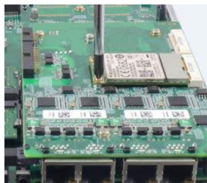
Secured with M2.5 P-head screw
