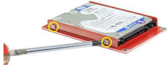
(HDD bracket of Nuvo-5000LP)
