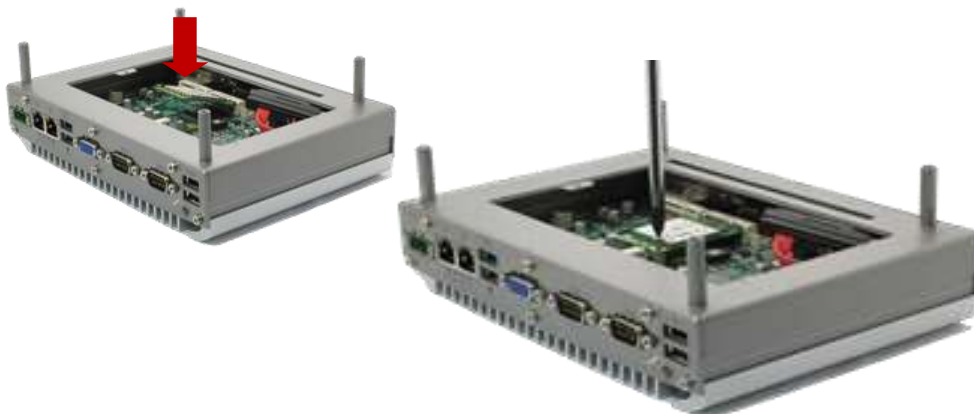
Figure 54: Install and Lock the Mini-PCle Module
