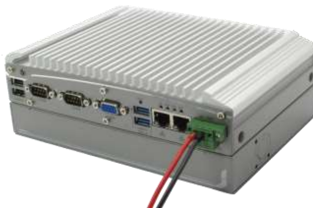
Figure 66: System with DC Input Terminal Block
