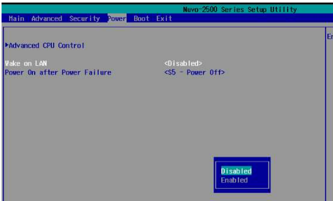
Figure 74: Enabling Wake on LAN in BIOS
