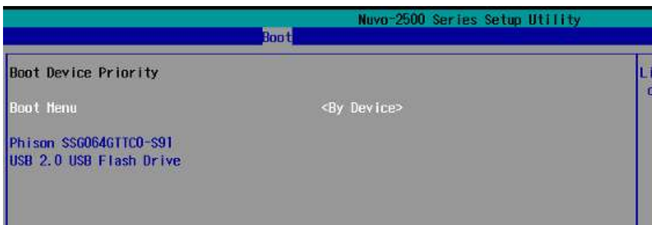
Figure 77: Configuring order of booting devices in BIOS
