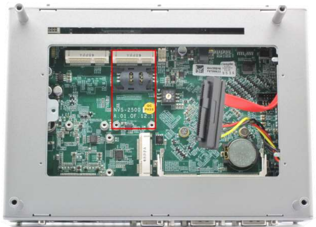
Figure 19: Mini PCI Express Connector and Internal SIM Socket
