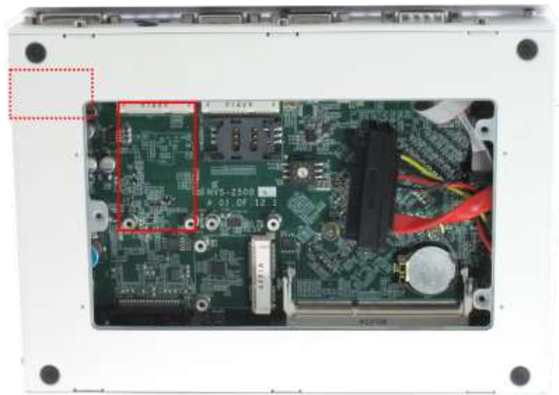
Figure 21: Mini PCI Express Connector with only USB Signal and External SIM Socket
