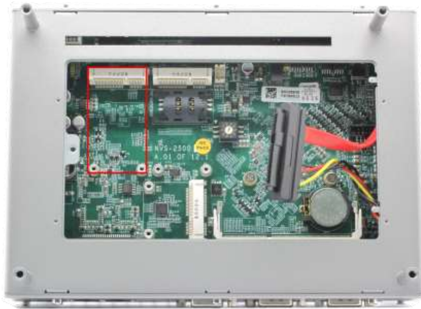
Figure 20: Mini PCI Express Connector with only USB Signal
