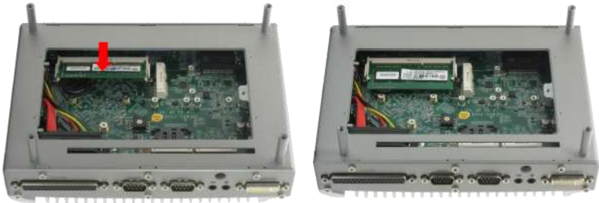
Figure 48: Install the Memory Module
