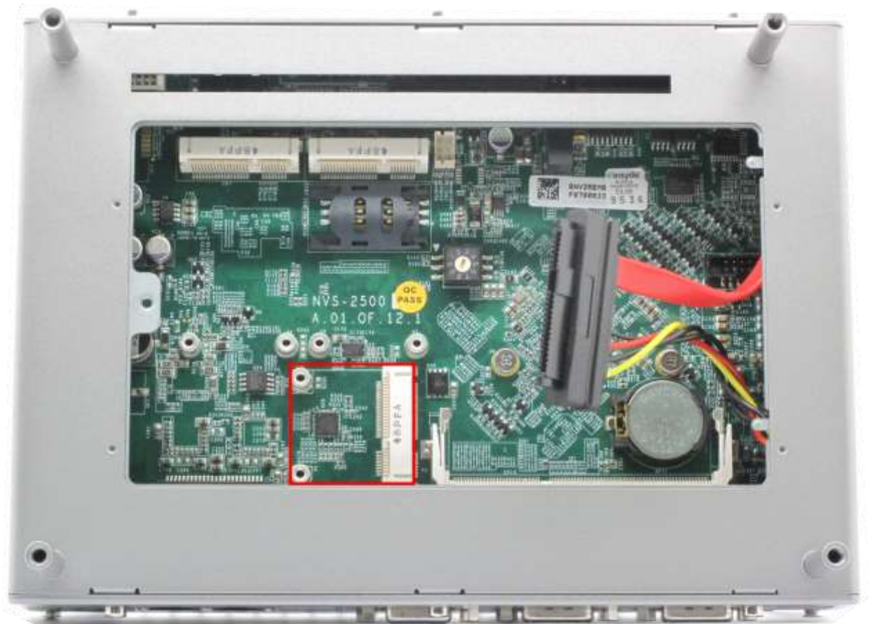
Figure 22: mSATA Connector with USB Signal
