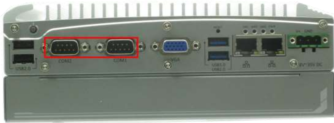
Figure 10: Software-programmable COM Ports
