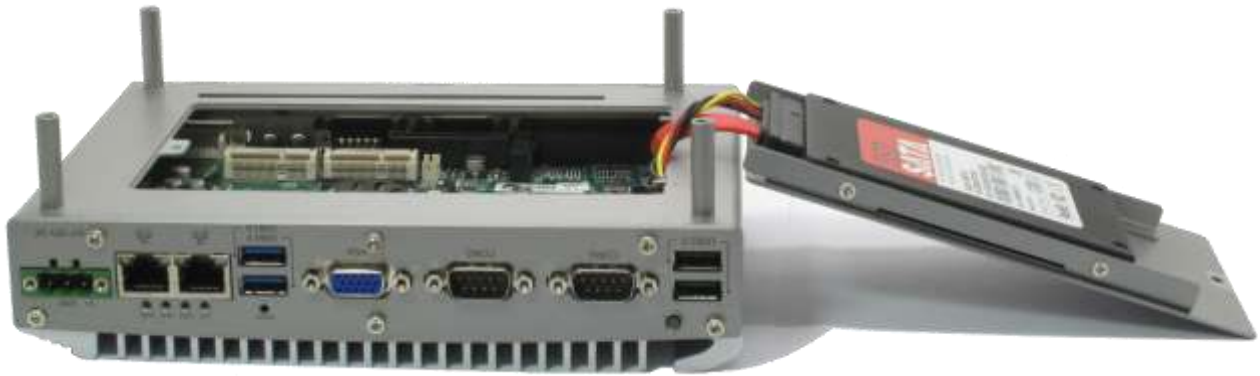
Figure 51: Connect HDD to the SATA Cable
