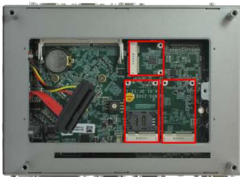
Figure 53: Mini-PCle and mSATA Connectors
