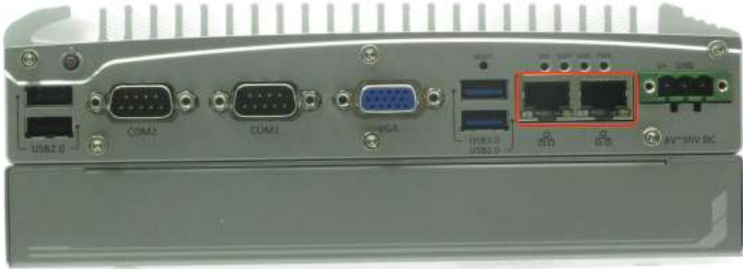
Figure 7: Nuvo-2500 Gigabit Ethernet Ports
