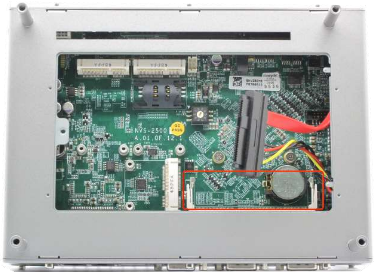
Figure 23: DDR3L SODIMM Socket
