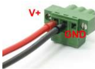
Figure 65: Wiring of DC Input Terminal Block
