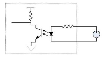
Figure 61: Wiring of isolated digital inputs
