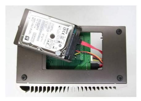
Figure 36: HDD bracket assembly connected to SATA cable
