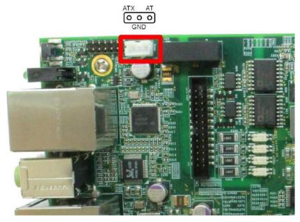
Figure 19: Remote on/off control connector
