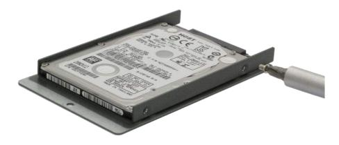
Figure 35: HDD bracket assembly of SATA connector #2
