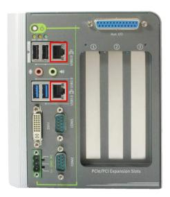
Figure 4: Gigabit Ethernet Ports
