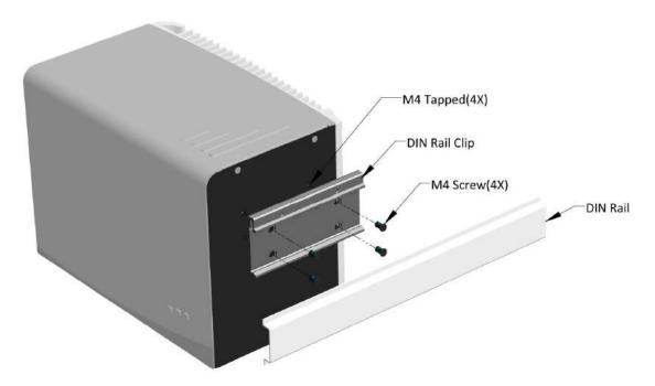
Figure 41: Assembling the DIN rail mounting clip
