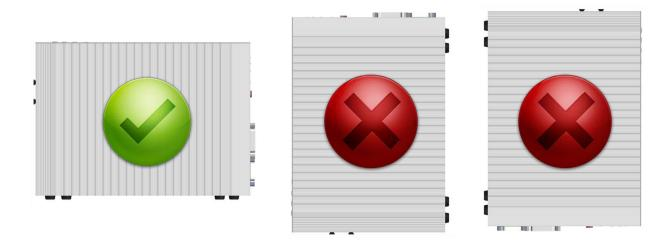
Figure 38: Correct Orientation of Mounting your System
