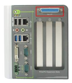
Figure 10: Isolated DI/O connector
