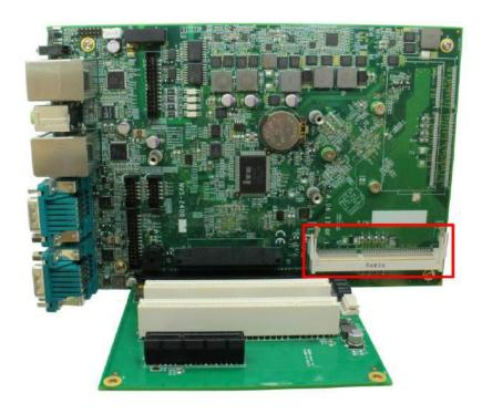
Figure 15: DDR3L SODIMM socket
