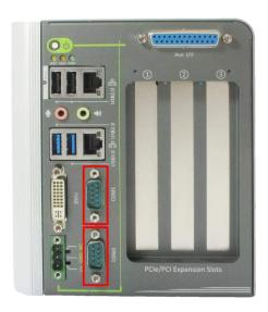
Figure 6: Software-programmable COM ports
