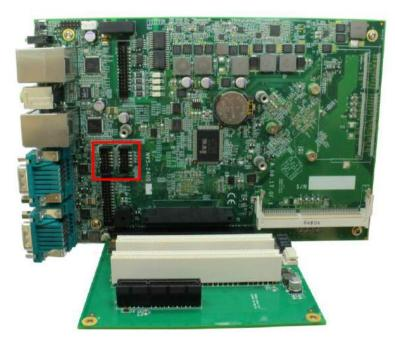
Figure 12: Internal COM ports
