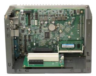
Figure 30: Install the memory module
