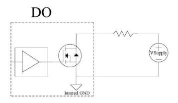
Figure 62: Wiring of isolated digital outputs
