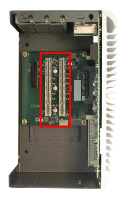
Figure 21: PCI Slots of Nuvo-2430(left) and Nuvo-2421(right)
