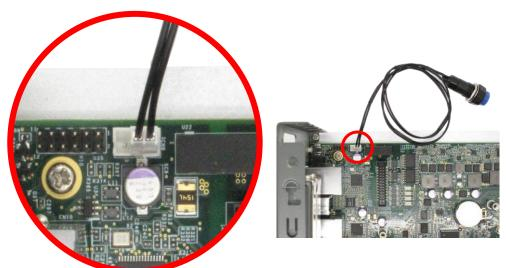
Figure 46: Connecting a latched switch to AT mode pin
