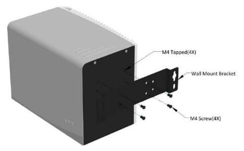
Figure 39: Assembling wall-mount bracket on the back side
