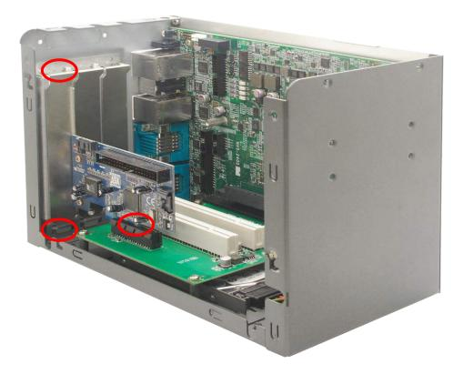
Figure 29: 3-point fixation of a PCI/PCIe card
