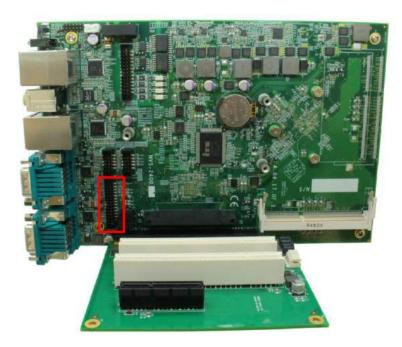
Figure 13: Internal parallel port
