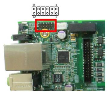
Figure 18: Remote status output connector
