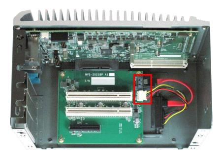
Figure 33: SATA cable connected to SATA connector #2
