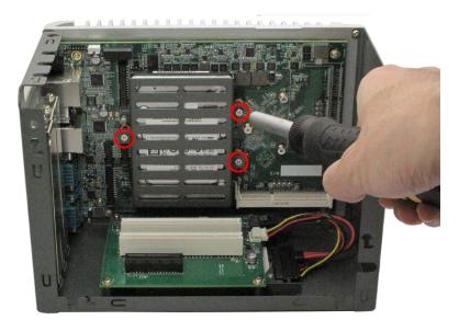
Figure 32: Installed HDD bracket assembly
