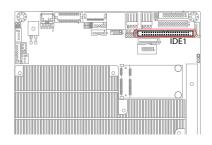
Consult the documentation that came with your IDE drive for details on jumper locations and settings. You must orient the cable connector so that the pin 1 (color) edge of the cable corresponds to pin 1 of the IDE connector.
