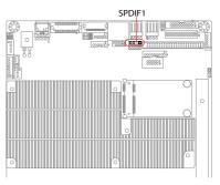
Check the pin assignment carefully while you connector the S/PDIF cable, incorrect connection between the cable and connector will make the device unable to work or even damage it. For optional S/PDIF cable, please contact your local dealer.
