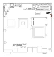
You may need to clear the CMOS if your system cannot boot up because you forgot your password, the CPU clock setup is incorrect, or the CMOS settings need to be reset to default values after the system BIOS has been updated. Refer to the following steps to reset your CMOS setting:
