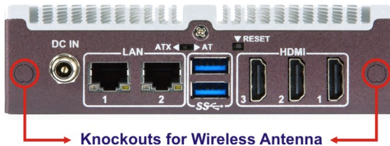
Figure 3-4: Knockouts for Wireless Antenna
