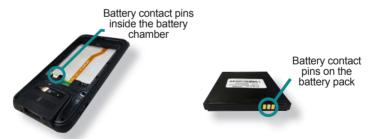
Place the battery into the battery chamber by an angle the contact pins can meet.
