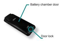
2. Use a coin to loosen the screw on the battery chamber door.
