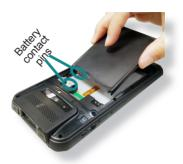
4. Snugly fit the battery inside the battery chamber.
