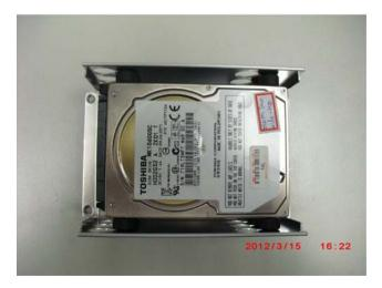
Step 3: Fasten the four screws to lock the HDD bracket and connect the SATA and power cable
