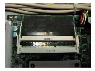
Step 6: Install the second SODIMM to the upper layer of memory slot
