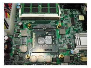
Step 2: Cover the CPU bracket and fasten the four screws to fix the CPU bracket, and then stick the thermal pad on the bracket
