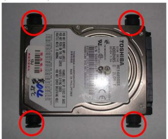
Step 4: Put the HDD back to the HDD bracket and lock the dampers
