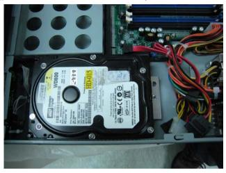
Step 5: Fasten the hard disk driver bay by using the screws
