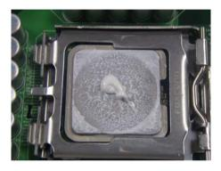
c. Place the Heatsink on the top of CPU. Please make sure that the four screws are aligned with the holes on the board.
