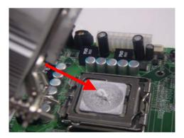
d. Fasten the four screws. First fasten the two screws (yellow) and then fasten the two screws (red) in sequence to secure the heatsink in place.
