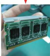
3. Attach another piece of heatsink to the SO-DIMM and hold them tight. Make sure the two pieces are aligned properly so that their notches can meet.
