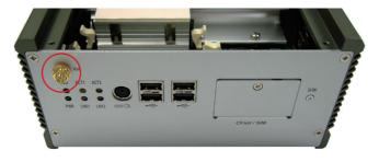
6. At the end, screw antenna into the SMA connector jack and adjust antenna angle for better signal.
