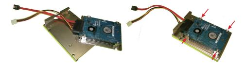
3. Plug power and SATA lines in corresponding PWR2 and SATA2 connectors. If you want to remove the 2nd HDD afterwards, press the metalic clip and pull off the white plastic clip to unplug the two lines.
