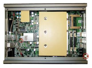
4. Push the plastic plug outwards to remove it, so that another end of RF cable, which is a SMA connector jack, can penetrate through antenna hole located on front pane. Keep the plastic plug for later use. When you try to penetrate the SMA connector jack through antenna hole, be sure to put the flat side (in red frame) rightwards, or it'll get stuck.
