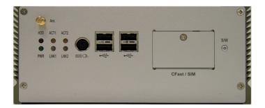
5. Mount a round washer into the SMA connector jack from outside before securing another nut into it.
