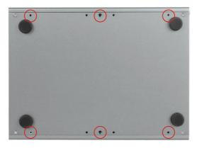
2. Use screwdriver to remove the bottom cover screws and keep them safely for later use.
