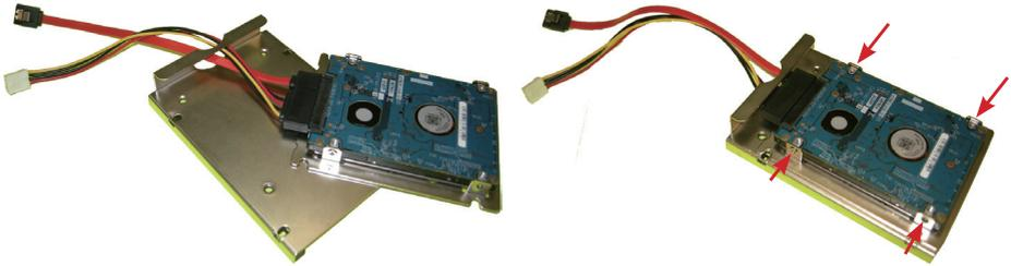
3. Plug power and SATA lines in corresponding PWR2 and SATA2 connectors. If you want to remove the 2nd HDD afterwards, press the metallic clip and pull off the white plastic clip to unplug the two lines.
