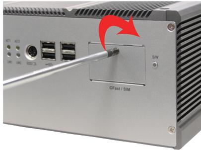
6. To remove the CFast card or SIM card, follow step 1, 2 and 3 above. And then push card inward to pop-out it from the slot.
