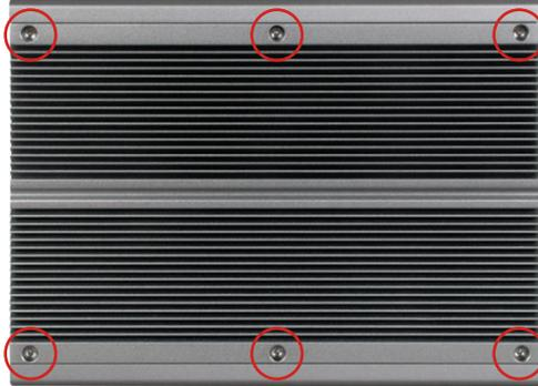
2. Use a screwdriver to remove top cover screws. First unscrew the four screws in each corner, and then two screws in the middle of two sides. Keep these screws safely for later use. (Remember to first secure two screws in the middle and then four corners when you are to install the top cover.)
