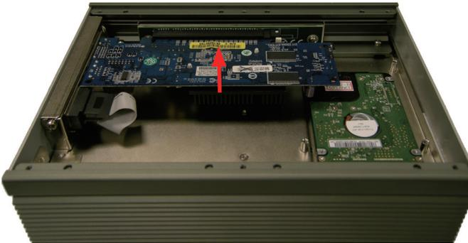
2. For 7512, follow the same procedure to install the upper PCIe card.
