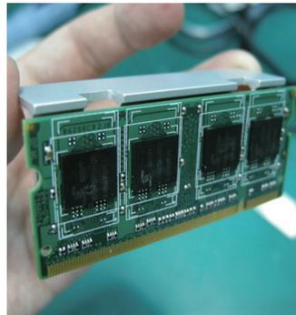
3. Attach another piece of heatsink to the SO-DIMM and hold them tight. Make sure the two pieces are aligned properly so that their notches can meet.
