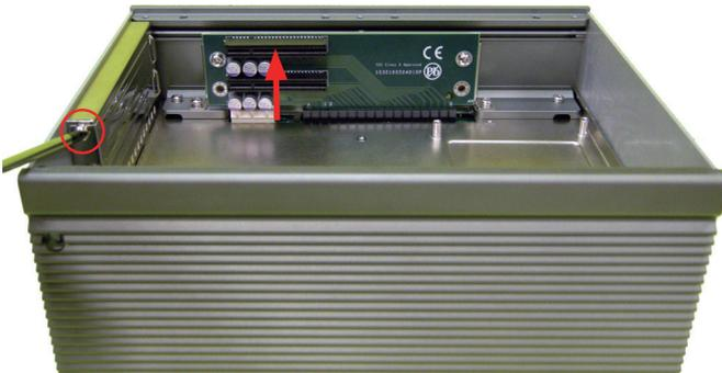
3. And penetrate through the hole on case side with screwdriver to remove lower bracket and install PCIe card.
