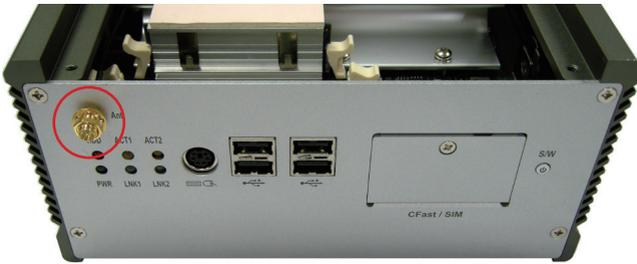
6. At the end, screw antenna into the SMA connector jack and adjust antenna angle for better signal.
