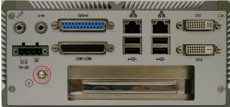
1. As the figure illustrates above, remove the ground screw located on the bottom-left of the rear panel.
