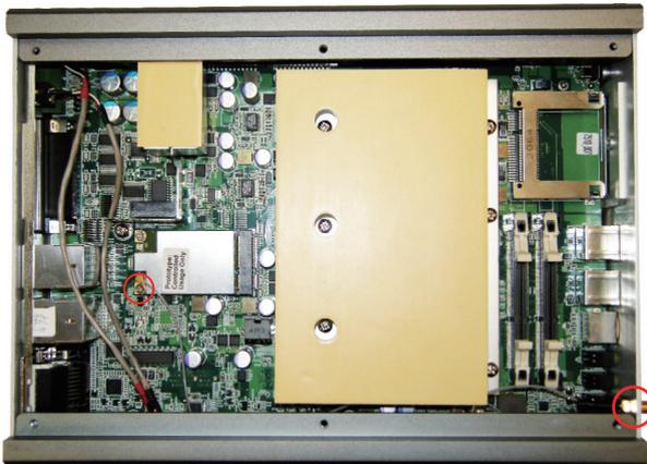
4. Push the plastic plug outwards to remove it, so that another end of RF cable, which is a SMA connector jack, can penetrate through antenna hole located on front pane. Keep the plastic plug for later use. When you try to penetrate the SMA connector jack through antenna hole, be sure to put the flat side (in red frame) rightwards, or it'll get stuck.
