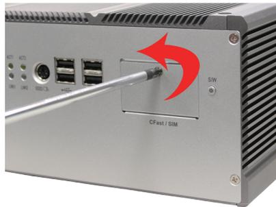
4. Insert your CFast/SIM card into the slot according to the illustration that you find close to the card holder.
