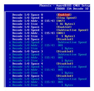
It allows you to use the IT8888 ISA Decode IO menu to set the IO memory range for the onboard ISA.
