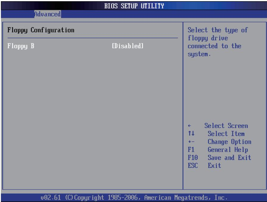
Select the type of floppy disk drive installed in your system.
