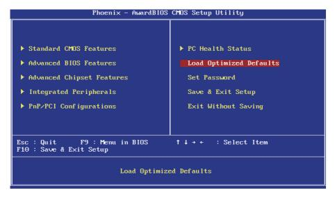
It allows you to load the default values to your system configuration. The default setting is optimal and enabled all high performance features.
