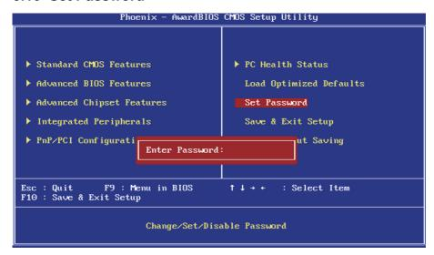
Using Password to set a password that will be used exclusively on the system. To specify a password, highlight the type you want and press <Enter>.
