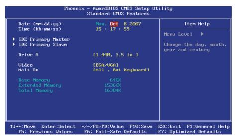
"Standard CMOS Features" allows you to record some basic hardware configurations in your computer system and set the system clock and If the handling. CPU card is already installed error need will this working system, you not to select option. You will need to run the Standard CMOS option, however, if you change your system hardware configurations, such as onboard battery fails, or the configuration stored in the CMOS memory was lost or damaged.
