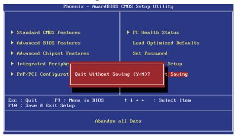
Typing "Y" will quit the Setup utility without saving the modifications. Typing "N" will return you to Setup utility.
