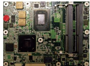
2. For COM-873E-827E, you have to put an additional thermal pad between heatsink and CPU module, but COM-873E-2610UE can skip this step. Please tear protective membranes on both sides from thermal pad first of all, be sure not to pinch or mold the thermal pad, and then put it as right picture.
