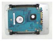
4. Fasten the two HDD brackets on the HDD cover with four screws
