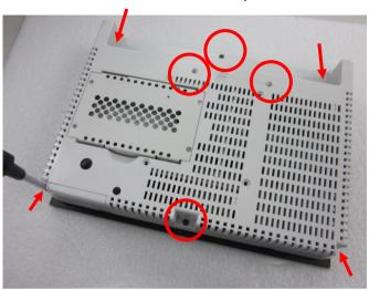
Step 2: Unfasten the three screws to take out the heat sink from AHP-1122
