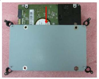
Step 4: Fasten the four screws to fasten the HDD and HDD backet
