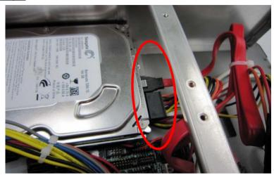
Step 4: Connect the SATA cable to the main board
