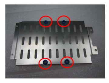
Step 4: Fasten the four screws to fix the bracket and HDD
