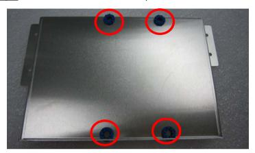
Step 2: Fasten the four screws to fix the bracket and HDD
