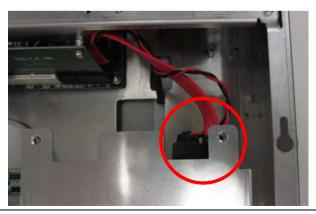
Step 3: Fasten the four screws to fix the DVD-ROM bracket with AGP-3155
