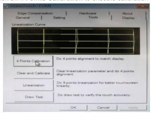
**Note:** If the alignments do not match display by 4 Points Calibration, please use 9 Ports or more to calibrate.
