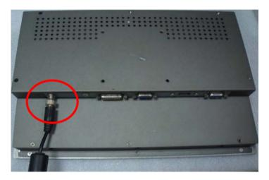
A "Surge Protection" device plugged between the AC-DC adapter and the wall outlet is recommended to prevent the effects of sudden current variations from reaching the LCD Display. The sudden peaks of electricity may harm the LCD Display.
