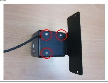
Step 2: Fasten the two screws (2-SELF TAPPING SCREWS) to fix the Bar Code Scanner with the ACP-5215
