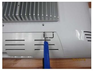
**Note 2:** The "Anti-Drop Kit" can help on preventing the cable drop from the connector
