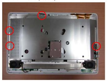
Step 3: Remove HDD Bracket (4 screws)
