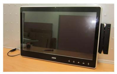
Step 1: Fasten the two screws (2-SELF TAPPING SCREWS) to fix the MSR Bracket with the ACP-5215
