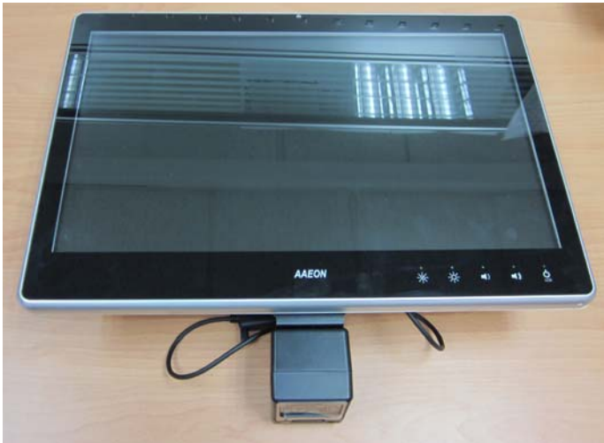
Step 1: Fasten the three screws to fix the Bar Code Scanner with the
